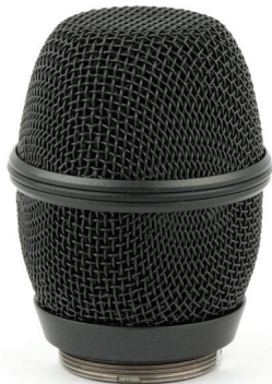
HHVMC Lectrosonics cardioid electret with VariMic preamp
