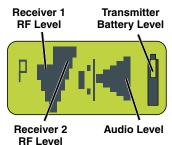
and mode selections. In the ratio diversity mode, the Main Window displays audio levels, transmitter battery status, pilot tone status and RF level activity for both receivers, with a single audio channel display.
