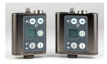
To meet the demand for both extended operating range and extended battery life, the "WB" series SM transmitters offer selectable output power of 25, 50 and 100 mW. With higher power output, the operating range is improved at the expense of battery life. When range is not an issue, a lower power level can be used to extend the battery life.
