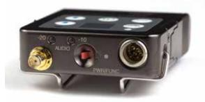
The housing is constructed of solid machined aluminum for lasting ruggedness. The exterior is finished with an ultra hard, black electroless nickel finish.
