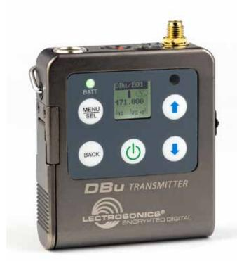
The DBu transmitter is a second generation design with specially developed, high efficiency digital circuitry for extended operating time on two AA batteries. The transmitter can tune in coarse or fine steps across the UHF television band from 470.100 to 607.950 MHz, with a selectable output power of 25 or 50 mW. The pure digital architecture enables AES 256-CTR encryption for high level security applications.
