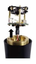
6) Set new capsule assembly to align the holes for the socket head bolts
