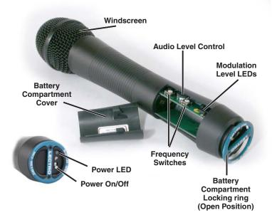
NOTE: A NiMH battery gives little or no warning when it is depleted. If you use NiMH batteries in the UT, we recommend trying fully charged batteries first, noting the length of time that the batteries will run the unit and in the future use somewhat less than that time to determine when the battery needs to be replaced.
