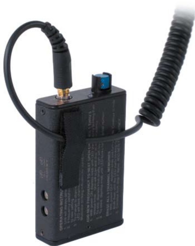
Figure 2 - Headphone cord strain relief
