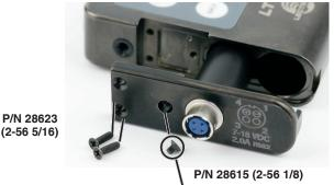
CAUTION: Use only the shorter screw P/N 28515 (2-56 1/8 in.) in the hole near the connector. The longer screws may damage circuit board component.
