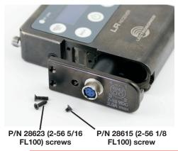
CAUTION: Use only the shorter screw P/N 28615 (2-56 1/8 in.) in the hole near the connector. The longer screws may damage a circuit board component.
