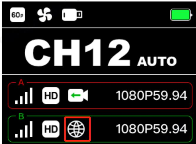
3. Long press the middle button of the receiver to enter the menu, select the "Streaming" function, and then select the "NDI".
