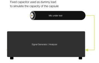
To simplify the process, many brands treat the **capsule** as an "ideal element" and instead focus on determining the maximum input level the amplifier can handle, hereby only measuring half of the microphone during the THD test. Thus, the THD value is measured as equivalent electrical input signal, which does not account for the contributions of the capsule or the interactions between the capsule and the preamp.
