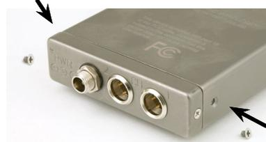
Panels are held in place by two Phillips head screws on the sides of the housing.
