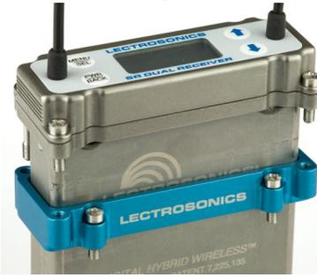
Thread two short screws through the recessed tabs on the adapter and slide it onto the receiver housing. Thread two short screws through the tabs on the receiver flange as shown.
