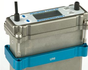
On the opposite side, thread two long screws through the tabs on the receiver flange, then align them with the tabs on the adapter.
