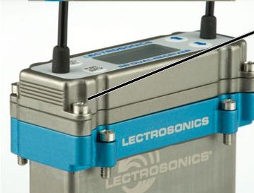
Slide the adapter up and tighten the retaining screws to secure it to the receiver flange.
