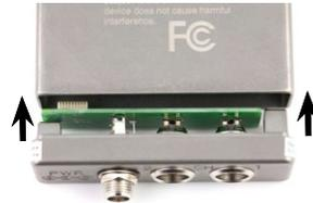
Carefully align the mating connectors and gently slide the panel straight into the housing until the screw holes align with the housing.
