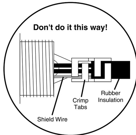
**Note:** This termination is required on VHF transmitters and will still work fine on UHF transmitters.
