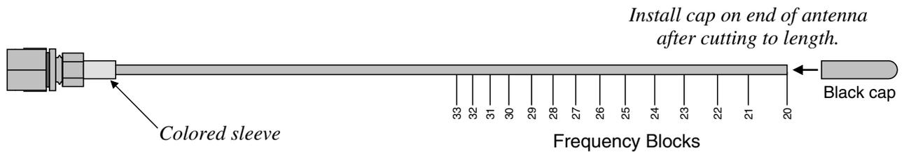
Kits are shipped from the factory with caps of the various colors plus a black cap. After cutting the antenna to the desired block length, select the properly colored cap and cut off the closed end to make the colored sleeve. Slide the colored sleeve onto the antenna as shown above then slide the black cap onto the cut end of the antenna.
