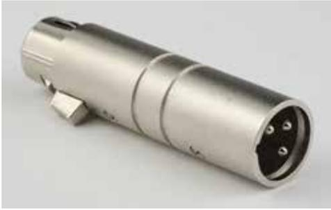
This polarity reversing adapter may be needed to correct for asymmetrical current draw in some P48 powered condenser microphones, including older Neumann 100 Series, Rode NTG3 and others. If your microphone does not power on correctly when used with HM, HMa and UH400a/TM transmitters, insert the adapter between the transmitter and microphone as shown.
