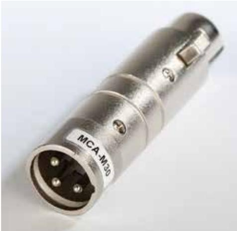
This adapter may be needed if you are experiencing noise or distortion with measurement microphones, particularly the Earthworks M30. The adapter has a common mode choke for suppressing RF noise. If your microphone signal exhibits these problems when connected to a HM, HMa and UH400a/TM transmitter, insert the adapter between the microphone and the transmitter as shown above.
