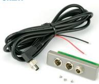
This kit includes an output and power panel with two TA3 male, balanced outputs and a power jack with a locking connector. A 6 foot power cable is included.
