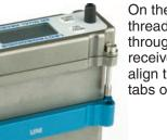
On the opposite side, thread two long screws through the tabs on the receiver flange, then align them with the tabs on the adapter.
