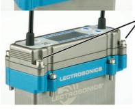
Slide the adapter up and tighten the retaining screws to secure it to the receiver flange.
