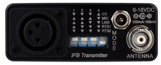
The rear panel provides the audio input and programming DIP switches for intercom and audio input type along with power and antenna input jacks.
