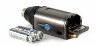
The battery compartment door is hinged to the housing and remains attached to the transmitter when opened. It latches securely in place and applies pressure to the batteries when closed. The two AA batteries are connected in series through a conductive plate on the door.
