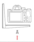
**Step #3** Mount camera and L-plate to tilt clamp.
