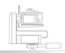
**Step #5** Plug in 12-24 volt power and immediately press and release the center PS button. Remote shows blue LED when connected.
