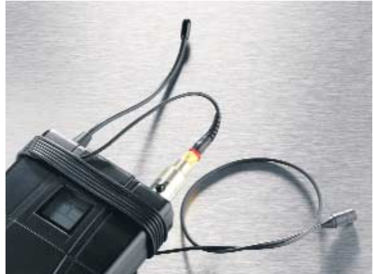
Correct way to wind up the cable of the Miniature Microphone. Please note the slack after the connector.
